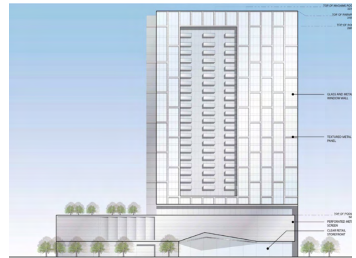
TOWER - SOUTH ELEVATION
