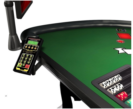
Figure 4: Installed Dealer Interface
